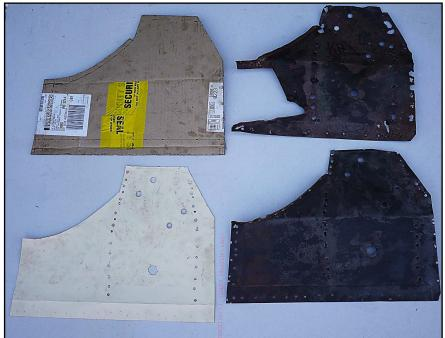
pearance [with varying degrees of enthusiasm]. To continue - basically patterns are, often, produced as a progressive series to the point where [for metal fabrication] a metal blank is produced and details transferred to the blank for finalising into a copy of an original item.
