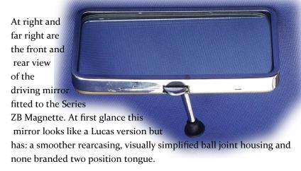
To emphasise how late in the production run this driving mirror is, it is fitted to Magnettes KAC 21/36,082 and KABJ 23/32,643.
